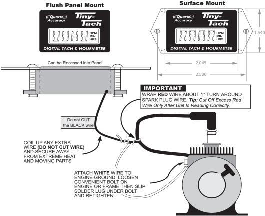
Wire damage (cuts or burns) will cause the wire to short and your *TINY-TACH*™ will stop working. *Wire damage is not* covered under warranty.
